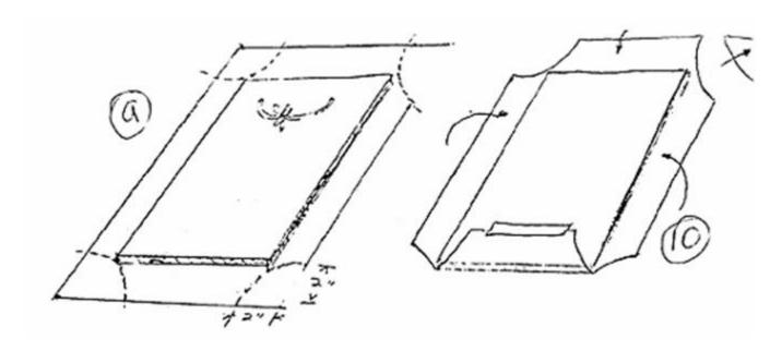
10. Fold the acetate one side at a time and tape as shown.
